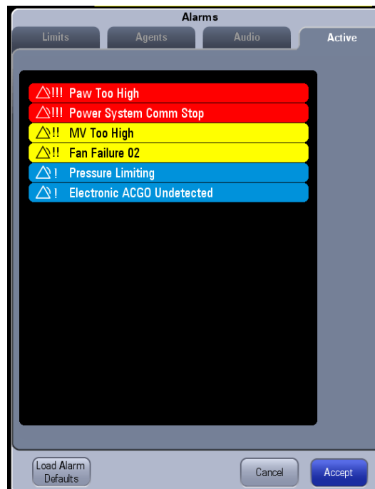
FIGURE 6-2 Active Alarms list in the Alarms window
