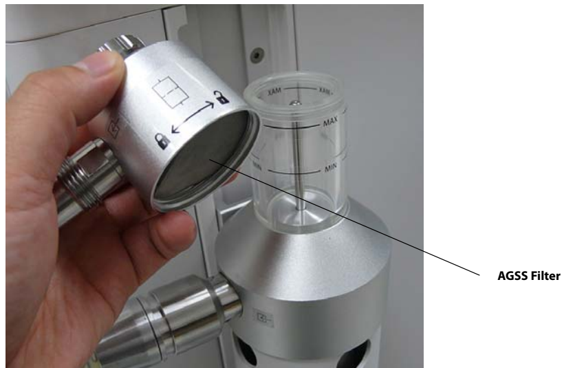
FIGURE 7-27 Removal of AGSS Top / AGSS Filter Inspection
