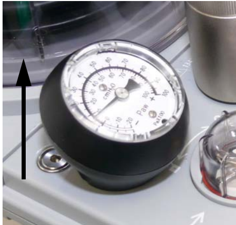
FIGURE 7-15 PAW Gauge Removal
