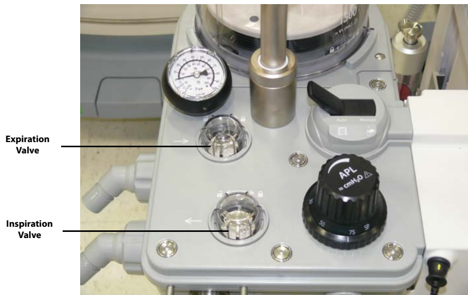
FIGURE 7-10 Location of Expiration and Inspiration Valves
