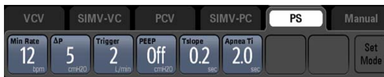
FIGURE 3-30 Ventilation Mode: PS
