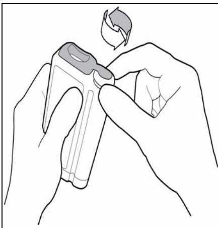
FIGURE 10-6 Removing Telepack-608 Battery Cap
