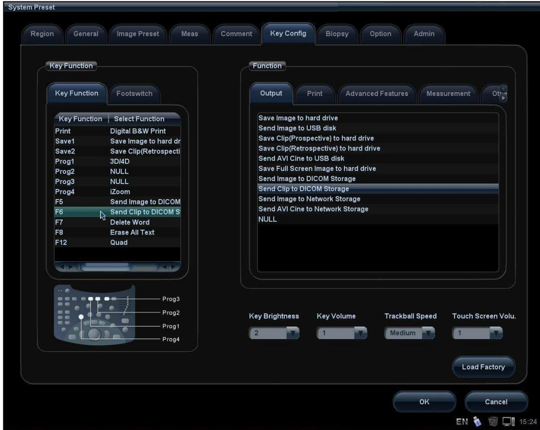
**Figure 15 Send to DICOM Storage by User-defined Key**
