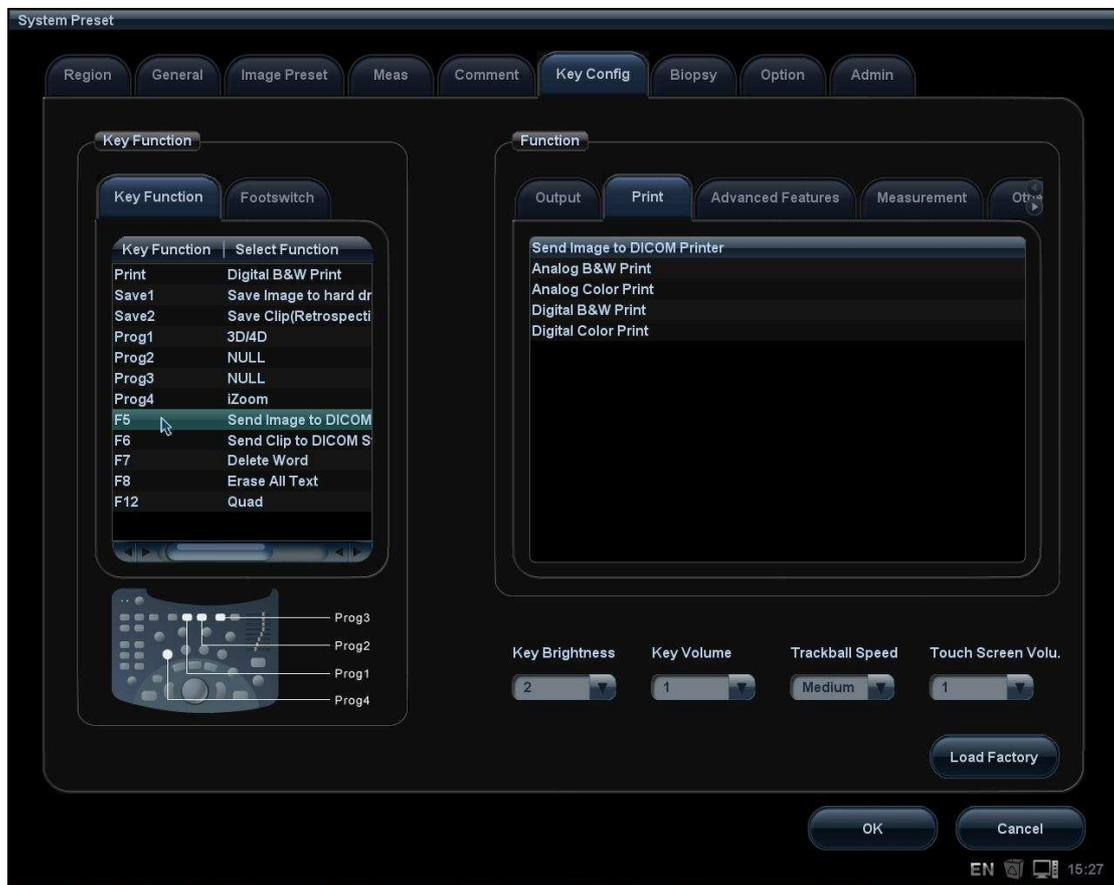
**Figure 17 Send to DICOM print when pressing user-defined key**
