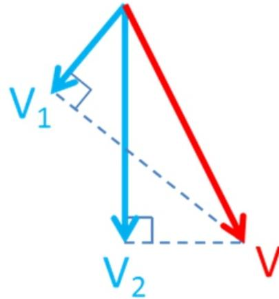
Fig. 3: Example for velocity obtained from two beams. Both the velocity and direction are obtained from an angle compounding technique, where  $V$  is the compounding velocity, and  $V_1$  and  $V_2$  are Doppler measured velocities.
