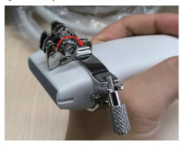
d. Select a suitable guiding block and loosen its nut, install the guiding block to the guiding block fixing frame and then tighten the block nut tightly.
