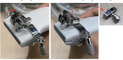
c. Rotate the clamping nuts on both sides of the needle guided-bracket to. separate The needle guided- the bracket is separate from the probe. Hold the probe and take it out of the bracket.
