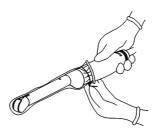
b. Align the needle-guided bracket with the probe to align the locating bulges on the needle guide with the locating grooves on the probe, then turn the retaining clamp to the correct position.
