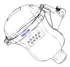
c. Tighten the pinch nut of the needle-guided bracket to confirm that the needle-guided bracket is properly installed on the probe. Loosen the angle adjusting nut.
