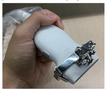
b. Loosen the guiding block nut, and remove it from the guiding block fixing frame.
