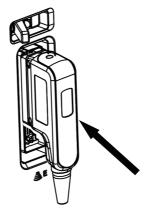
3. Pull down the tightening part of the probe adapter.
