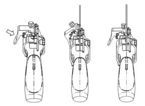
d. Hold the probe, and release the pressure position of the needle. Adjust the needle-shaped adjusting nut manually (following the direction of the arrow). The needle moves smoothly at the vertical direction due to its gravity.
