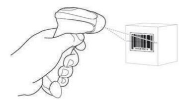
Do not hold the reader directly over the barcode. Laser light reflecting directly back into the reader from the barcode is known as specular reflection. This specular reflection can make
