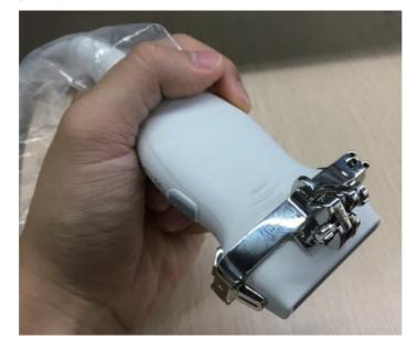
b. Loosen the guiding block nut, and remove it from the guiding block fixing frame.
