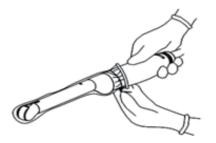
b. Open the retaining clamp, align the needle-guided bracket with the transducer to locate the locating bulge on the needle guide to the locating grooves on the transducer, and then turn the retaining clamp to match it with the transducer.
