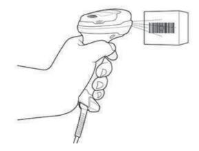
3. When the digital imager reader senses movement, in its default Auto Aim trigger mode, it projects a red LED dot which allows positioning the barcode within the field of view.
