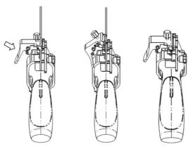
b. Rotate the locking nuts of the needle guided-bracket at the right and left sides (following the direction of the arrow). The needle guided-bracket is separate from the probe. Hold the probe and take out the bracket.
