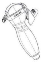
c. Rotate the clamping nuts of the guided bracket on right and left side to fix the bracket and the transducer. Rotate the needle-type adjusting nut to the ultimate position as shown in the figure.
