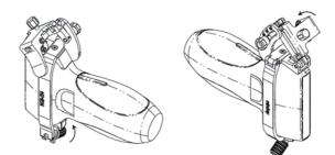
c. Hold the probe. Press the biopsy needle pressure position to separate it from the V-shaped guiding block. Put the needle into the V-shaped guiding block of the needle guided-bracket.
