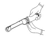
b. Align the needle-guided bracket with the probe to align the locating bulges on the needle guide with the locating grooves on the probe, then turn the retaining clamp to the correct position.
