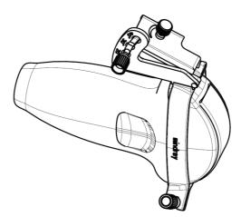
a. Hold the transducer. Press the pressure position of the needle to separate needle guided V-shaped block from pressure position of the needle.
