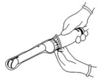
b. Open the clamp. Insert the front clamp to the front groove, and align front clamp with front groove.
