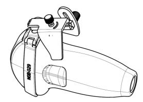
2. Tighten the fixing nut of clamps of the needle-guided bracket to confirm that the needle-guided bracket is properly installed on the probe. And tighten the pinch nut (following the arrow's direction).
