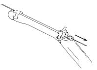
b. Hold the probe in one hand, and hold the bracket with the other hand. Press the separating button of the bracket to open the clamp.
