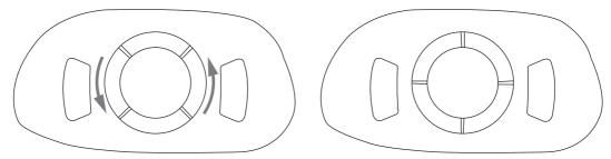
Put the ball in. Then, put the pressure ring in (the convex strip on the pressure ring is about 15 degrees from the horizontal), and rotate counterclockwise until the convex strip on the pressure ring is horizontal. Then, the buckle is locked. At this time, the pressure ring can no longer be rotated, indicating that the pressure ring has been installed in place.
