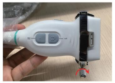
c. Loosen the depth pinch nut and fix it into the designated position of the depth shift sign after setting the desired depth.
