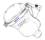
c. Tighten the pinch nut of the needle-guided bracket to confirm that the needle-guided bracket is properly installed on the probe. Loosen the angle adjusting nut.
