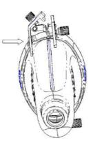
f. Release the pressing block, adjust the angle adjusting nut to confirm that the needle can freely slide in a vertical direction.
