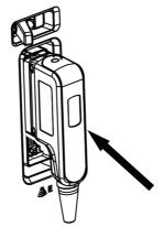
3. Position the probe properly to avoid it being treaded on or becoming wrapped around other devices. DO NOT allow the probe head to hang free.
