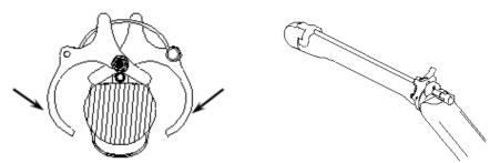
d. Hold the probe and insert the needle through the horn-shaped opening at the end of the bracket into needle guide.
