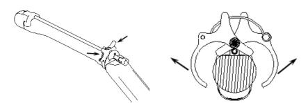
c. Hold the clasp at the end of the bracket to separate the bracket from probe.
