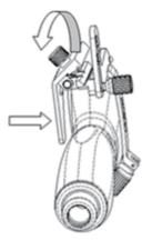
e. Put the needle into the needle guided-bracket, and the needle leans to V-shaped block.
