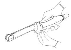
4. Inspect the sheath to ensure there is no hole or tear.
