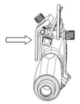
f. Hold the transducer, and release the pressure position of the needle. Adjust the needletype adjusting nut manually (following the direction of the arrow). The needle moves smoothly at the vertical direction due to its gravity.
