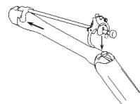
c. Arrange the probe sheath in order. Press the left and right clamps of the bracket to crosswise clamp the probe. Check if the bracket is properly installed to ensure that the it won't come off.
