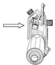
b. Separate the bracket and the transducer from the needle.
