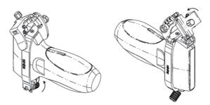
c. Hold the probe. Press the biopsy needle pressure position to separate it from the V-shaped guiding block. Put the needle into the V-shaped guiding block of the needle guided-bracket.
