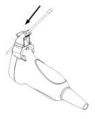
3. Release the needle from the bracket:
