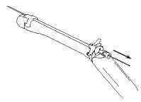
b. Hold the probe in one hand, and hold the bracket with the other hand. Press the separating button of the bracket to open the clamp.
