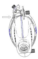
f. Release the pressing block, adjust the angle adjusting nut to confirm that the needle can freely slide in a vertical direction.
