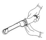
b. Open the retaining clamp, align the needle-guided bracket with the probe to align the locating bulge on the needle guide with the locating grooves on the probe, then turn the retaining clamp to align it with the probe.
