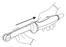
3. Secure the sheath with the enclosed elastic bands.
