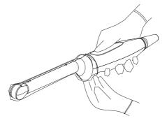
4. Inspect the sheath to ensure there is no hole or tear.
