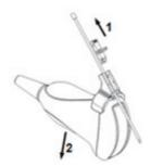
c. Remove the support of needle-guided bracket from the probe.
