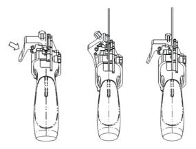
d. Hold the probe, and release the pressure position of the needle. Adjust the needle-shaped adjusting nut manually (following the direction of the arrow). The needle moves smoothly at the vertical direction due to its gravity.
