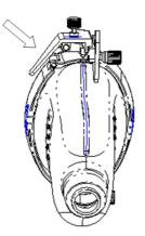
e. Insert the needle into V-shaped guided block.
