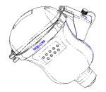
c. Tighten the pinch nut of the needle-guided bracket to confirm that the needle-guided bracket is properly installed on the probe. Loosen the angle adjusting nut.
