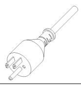
**NOTE:** Make sure to allow sufficient slack in the cable so that the plug will not be pulled out of the receptacle if the system is moved slightly. If the plug is pulled out accidentally, data may be lost.
