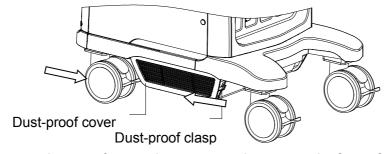
Probe port dust-proof cover: there are 4 probe ports at the front of the system, on which there is a dust-proof cover. Pull it out.
