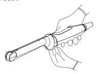
(2) Open the retaining clamp, align the needle-guided bracket with the probe to locate the locating bulge on the needle guide to the locating grooves on the probe, and then turn the retaining clamp to match it with the probe (See the figure below).
