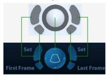
The left/right kidney shaped key is the <Set> key, to confirm the operation, similar to the left-button of the mouse. Press to confirm an operation, same as the left-button of a mouse.
