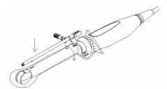
(3) When the retaining clamp is turned to the right position, the locking nut will lock the retaining clamp and the needle-guided bracket is then mounted to the right position.
