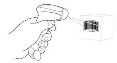
Tips: Do not hold the reader directly over the barcode. Laser light reflecting *directly* back into the reader from the barcode is known as specular reflection. This specular reflection can make decoding difficult. You can tilt the reader up to 55 forward or back and achieve a successful decode
