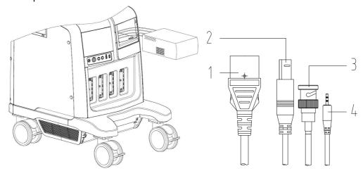
• Color analog video printer: use the I/O panel at the rear side of the machine to connect the printer, as shown in the following figure:
