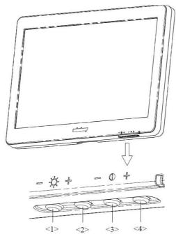
**NOTE:** On the monitor, the brightness adjustment comes before contrast. After readjusting the monitor's contrast and brightness, adjust all preset and peripheral settings.
