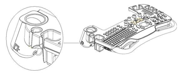
As shown in the figure above, the warmer is installed at left side of the control panel, the position that is used for placing the ultrasound gel.
