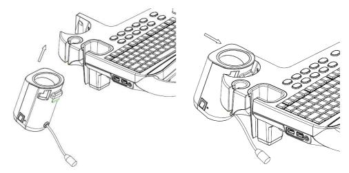
2. Push the warmer as per the arrow direction until it is tightly fixed, and connect the power cable to the power socket under the control panel.
