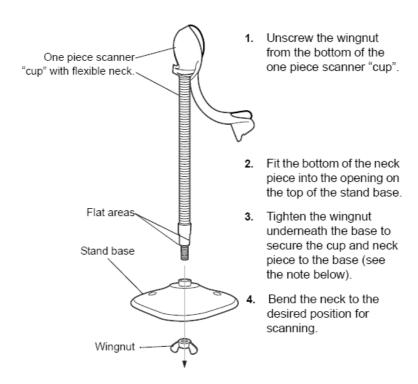
**NOTE:** Before tightening the wingnut under the base, ensure that the flat areas on the flexible neck fit securely in the grooves in the base.
