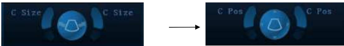
In current status, the trackball is used for adjusting ROI position
