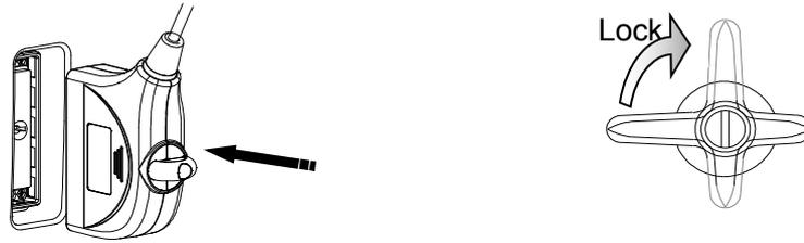
**NOTE:** Before inserting the connector into the probe port, inspect the connector pin. If the pin is bent, do not use the probe until it has been inspected / repaired / replaced.
