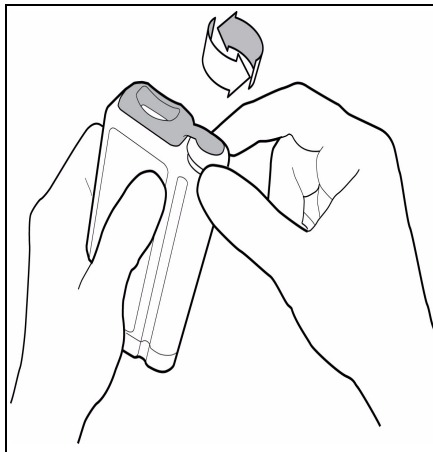
FIGURE 10-6 Removing Telepack-608 Battery Cap
