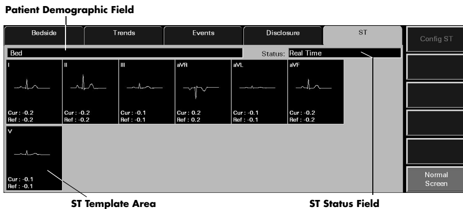
FIGURE 7-25 ST Tab - Hardwired Bedside Monitor (5-wire lead set)
