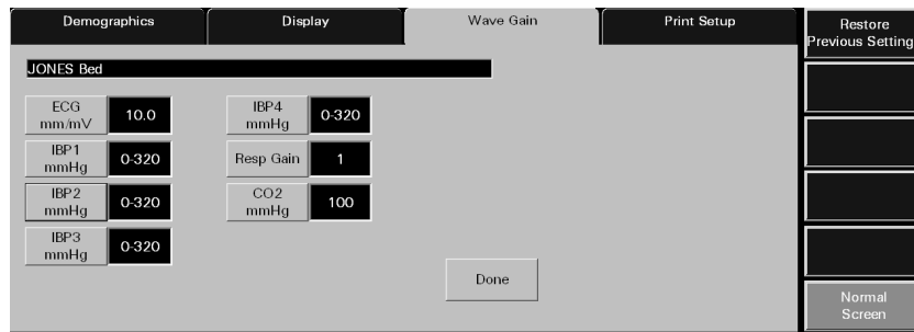
FIGURE 5-34 Wave Gain Tab (ViewStation and WorkStation)
