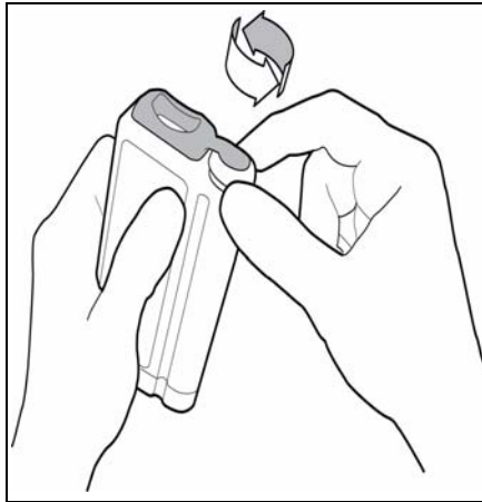
FIGURE 10-7 Removing Telepack Battery Cap
