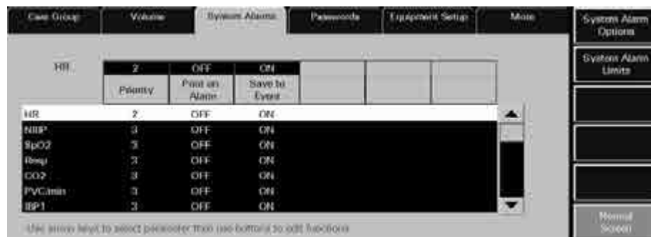
FIGURE 9-19 System Alarms (System Alarm Responses) Tab (Central Station)
