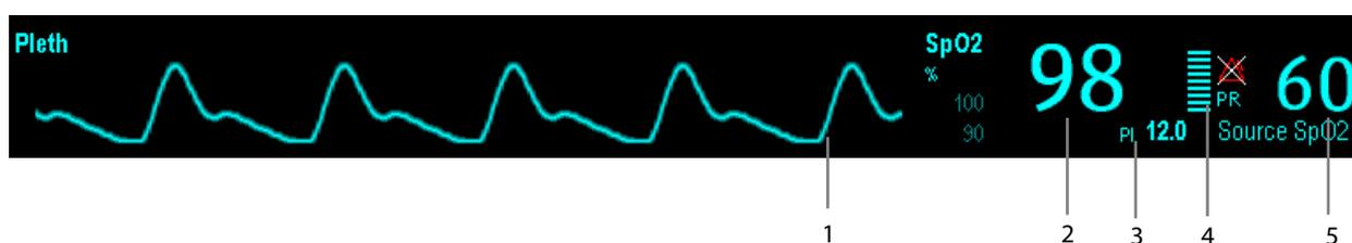
1. Pleth waveform (Pleth): visual indication of patient's pulse. The waveform is not normalized.
