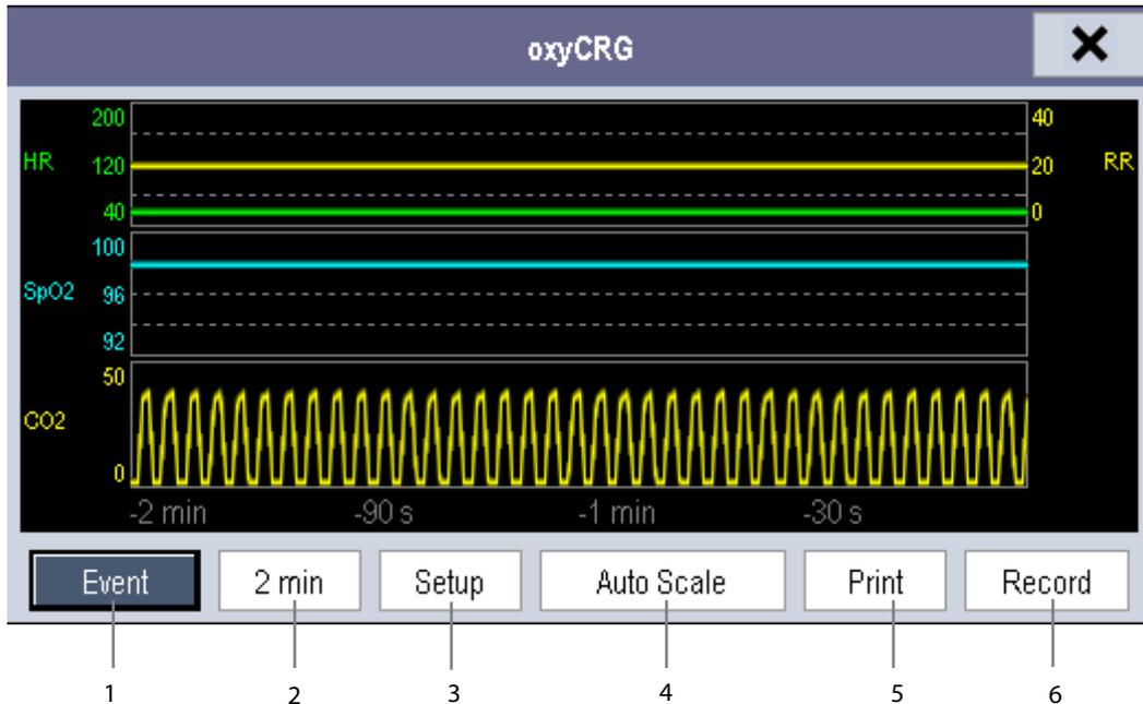
The split-screen view covers the lower part of the waveform area and shows HR trend, SpO<sub>2</sub> trend, RR trend, and a compressed wave (Resp wave or CO<sub>2</sub> wave). At the bottom, there are controls:
