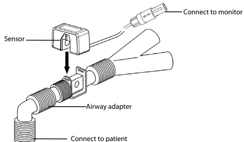
5. Make sure there are no leakages in the airway and then start a measurement.
