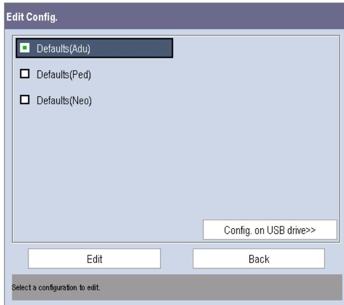
2. The popup menu shows the existing configurations on the monitor. Selecting [**Config. on USB drive >>**] will show the existing configurations on the USB drive. Select the desired configuration and then select the [**Edit**] button. The following menu appears.
