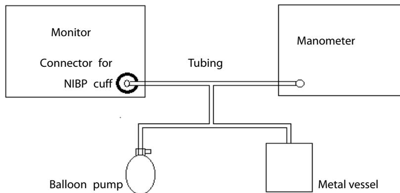
2. Before inflation, check that the reading of the manometer should be 0. If not, open the valve of the balloon pump to let the whole airway open to the atmosphere. Close the valve of the balloon pump after the reading is 0.
