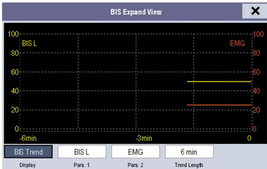
You can the desired trend lines to be displayed and set the time scale. The artifact mark is displayed at the bottom to indicate SQI value. When  $SQI < 15\%$ , the artifact mark is yellow and the corresponding trend lines of BIS, SR, BC and sBIS are not displayed. When  $15\% \leq SQI < 50\%$ , the artifact mark is brown.
