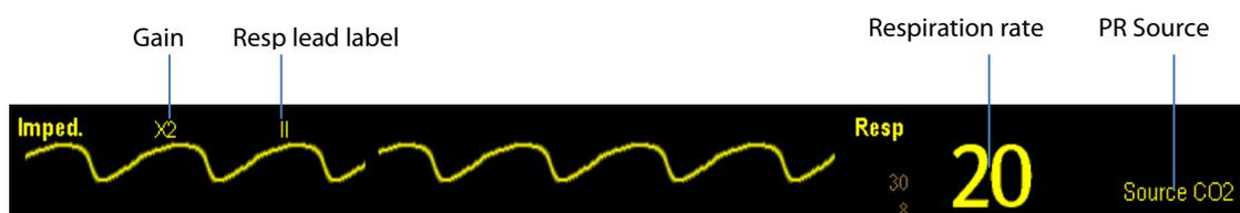
By selecting the waveform area or parameter area, you can enter the **[Resp Waveform]** menu. By selecting the Resp parameter window, you can enter the **[Resp Setup]** menu.
