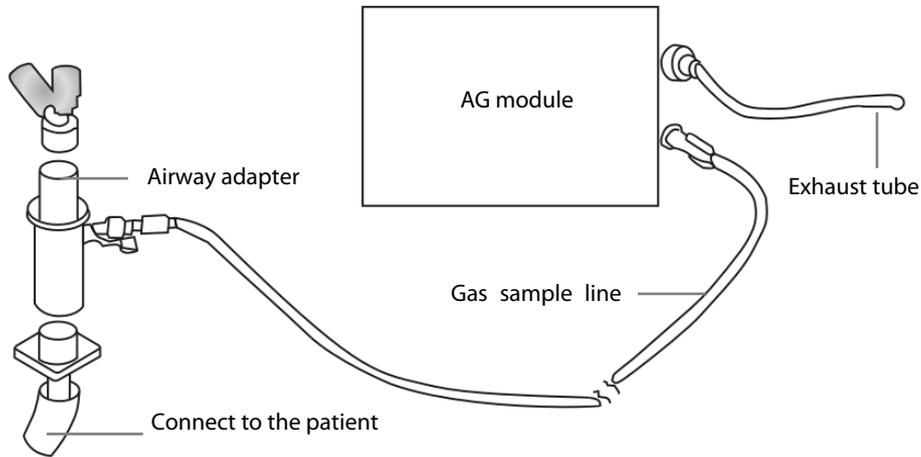
5. Insert the AG module to the patient monitor and the patient monitor will prompt **[AG Startup]**. Then the AG module starts to warmup and at the same time the patient monitor prompts **[AG Warmup]**. After 45 seconds, the AG module enters the iso accuracy mode. After 10 minutes, the module enters the full accuracy mode.
