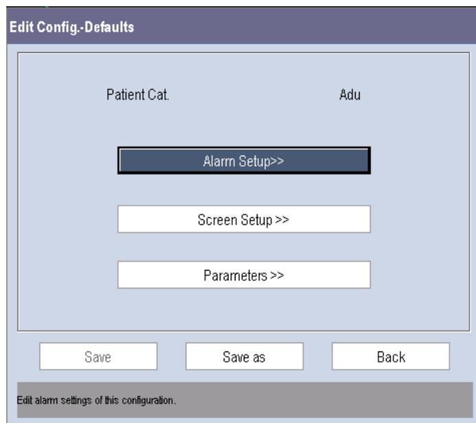
3. Select [**Alarm Setup >>**], [**Screen Setup >>**] or [**Parameter >>**] to enter the corresponding menu in which settings can be changed. The changed items of alarm setup will be marked in red.
