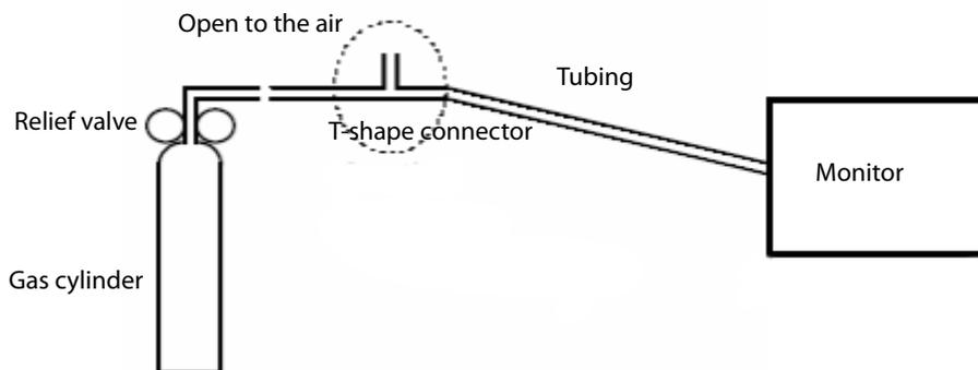
5. Open the relief valve and vent a standard gas and make sure that there is an excess gas flow through the T-shape connector to air. And wait for at least 30 seconds until the gas reading stable.
