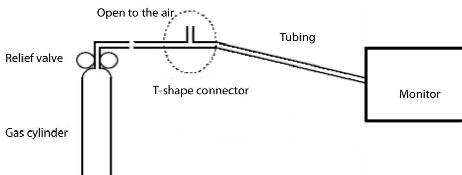
5. Open the relief valve to vent standard CO<sub>2</sub> and make sure that there is an excess gas flow through the T-shape connector to air.
