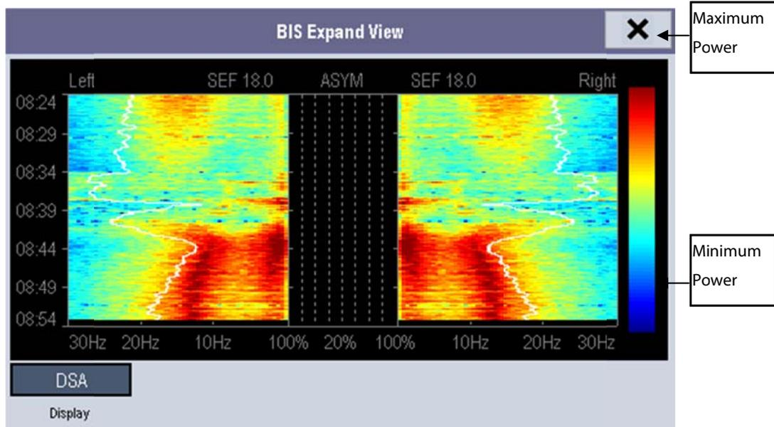
The Density Spectral Array (DSA) shows changes in the power spectrum distribution over a certain time period. The DSA represents the power spectra ranging from 49-94 dB. The color bar to the right of the time scale shows the range of colors used to indicate minimum and maximum power. The frequency scale is shown on the horizontal axis with a range from 0-30 Hz.
