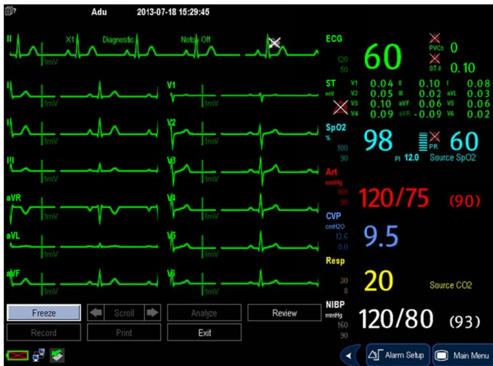
There are totally 12 ECG waves and 1 rhythm wave displayed on the screen. The rhythm lead is ECG I before entering the 12-lead ECG monitoring screen.
