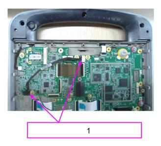
1 Unplug the keypad backup connectors from the two boards.
