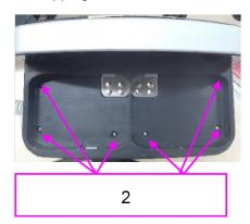
4. Gently lift the electrode base assembly upward, and unplug the cable plug connecting the electrode base from the in-position detection metal plate of the rear shell assembly. Replace the electrode base assembly.
