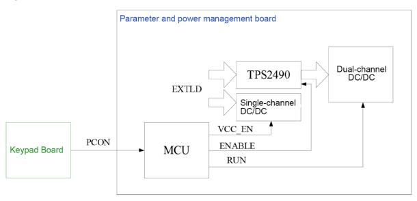
Power-on: Press the power key on the front panel of the equipment. The PCON signal changes from 1 to 0. The MCU wakes up, immediately outputs an ENABLE signal to TPS2490 to enable VBUS, enables the RUN signal of the dual-channel DC-DC module, and then outputs 5 V (VBB) and 12 V voltages.
