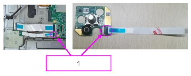
1 Disassemble the encoder FFC cable.
