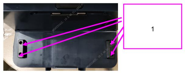
Four M3X12 cross recessed pan head screws with washers
