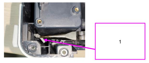
1 IO Port Silicon Plug of DX Host
