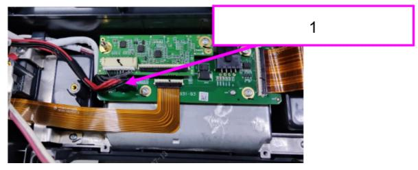
DC Input Cable of Defibrillator DX Power Parameter Board
