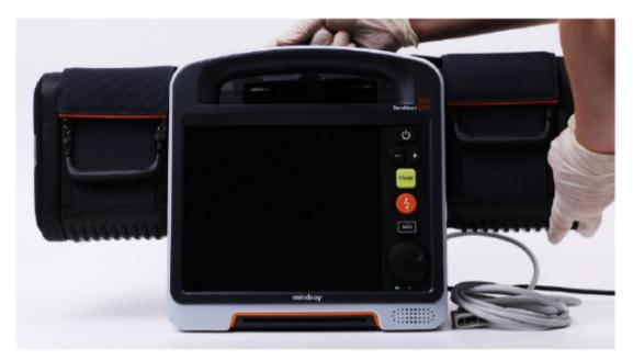
4. Click the icon in the upper right corner of the DX screen to confirm WIFI signal strength and Bluetooth signal strength. (When the distance between DX and N1 is within 1 meter, it is necessary to ensure that the Wi-Fi and Bluetooth signal strengths are greater than -65dBm)
