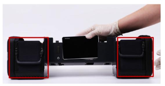
3. Put the N1 portable kit into the slot of the DX host, and the pairing will be completed automatically.
