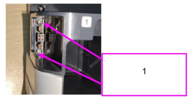
1 Two M2.5X12 cross recessed pan head screws
