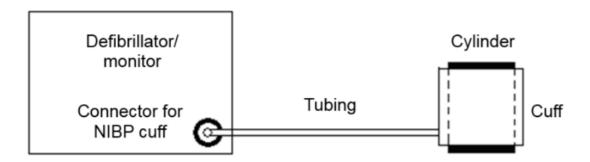
5. Enter the maintenance mode. Choose Module>NIBP>NIBP Leakage Test. After about 20 seconds, the equipment automatically deflates. This means the leakage test finishes. The leakage test is completed. The result is displayed on the screen. If the message "NIBP Pneumatic Leak" is displayed, it indicates that the NIBP airway may have leakage. Check the tubing and connections for leakages, and then perform a leakage test again.
