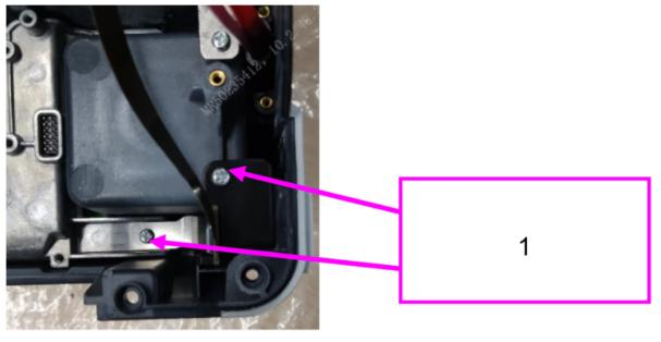
Two M3X6 cross recessed pan head screws
