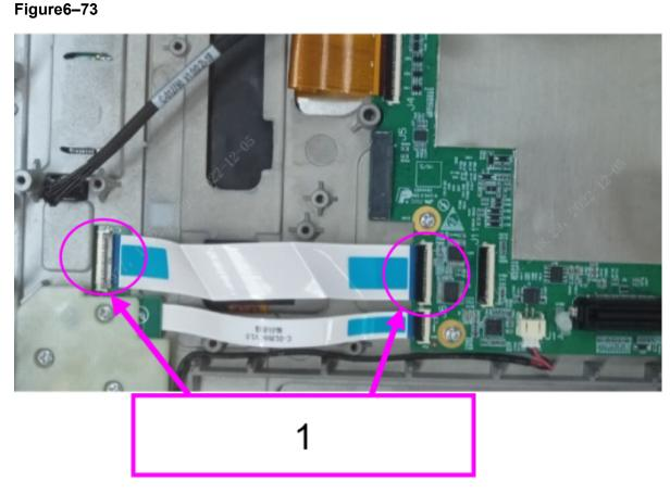
1 Disassemble the keypad FFC cable.
