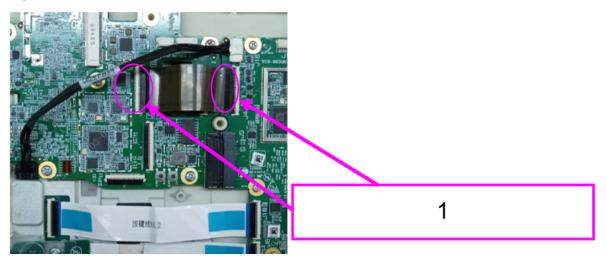
1 Remove the FPC cable connecting the slave board to the main control board.
