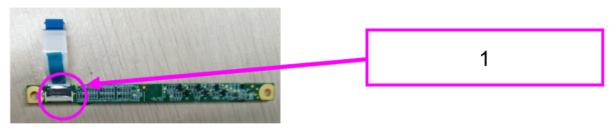
Disassemble the alarm LED FFC cable.
