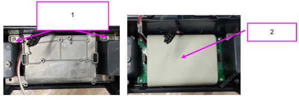
1 Two M3X6 cross recessed pan head screws
