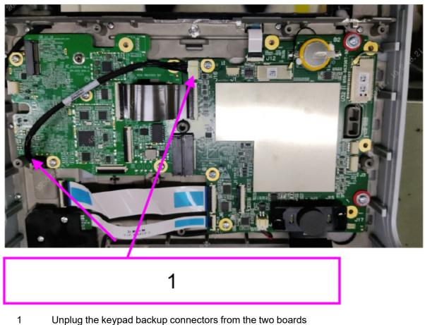
Unplug the keypad backup connectors from the two boards
