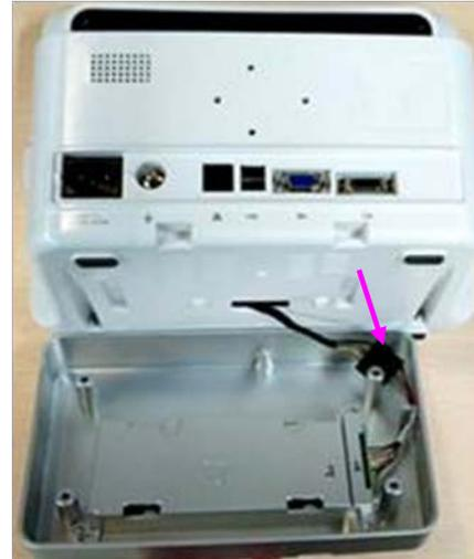
2. Remove the battery box component.
