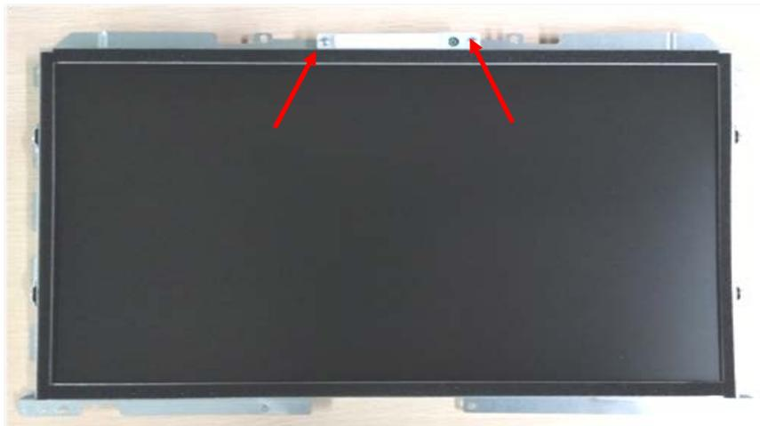
6. Loosen the two M3X6 screws with the mark "b" on the right top of the sheet metal.
