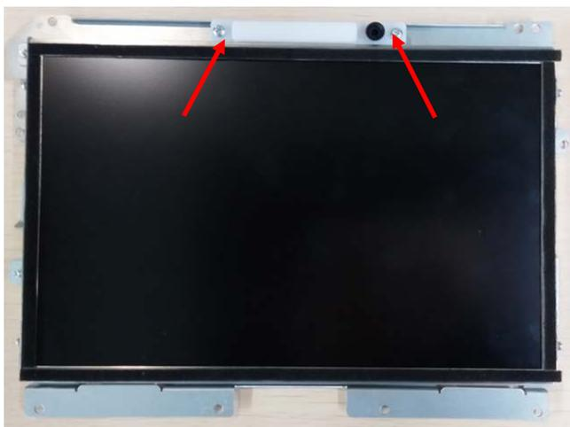
6. Loosen the two M3X6 screws with the mark "b" on the right top of the sheet metal.
