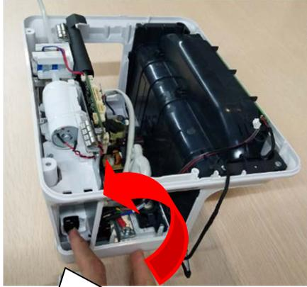
After the battery is switched to the vertical position, close the battery cover.
