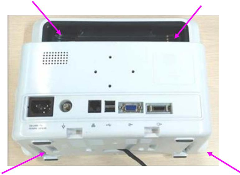
2. Open the front/rear housings, and remove the display screen connection cable and keypad connection cable.
