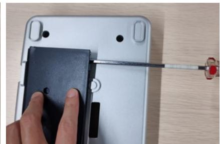
4. Use the Phillips screwdriver to loosen two M3X6 screws, take the bracket fixing the battery adapter out, use the Phillips screwdriver to loosen two M3X6 screws, and take the battery adapter out.
