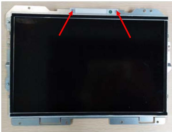
6. Loosen the two M3X6 screws with the mark "b" on the right top of the sheet metal.
