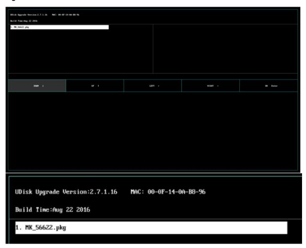
If the USB Flash disk just contains the upgrade kit file, the file is selected by default. If multiple upgrade kits are available, up to 16 kits are displayed in two columns. You can press the direction key to select the target upgrade kit.
