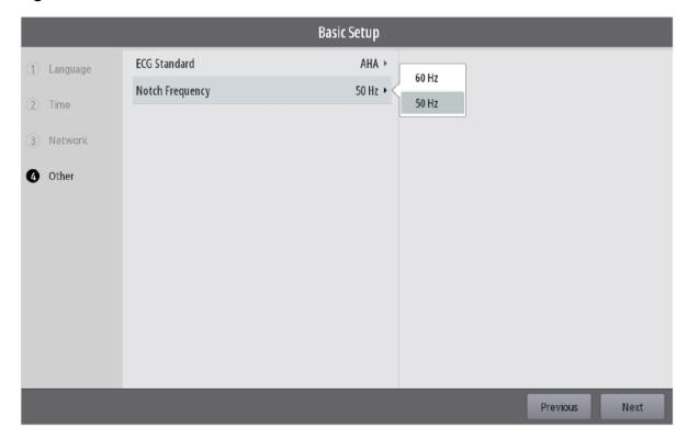
After completing the setup wizard, restart the ECG machine to finalize the settings and apply the changes.
