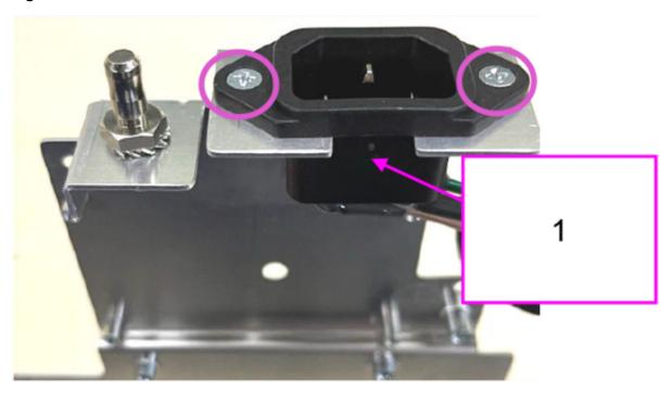
1 Connect the AC input wire to the main sheet metal.
