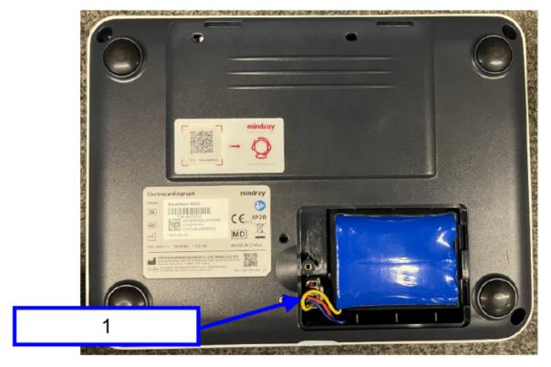
1 Loosen the battery cable buckle
