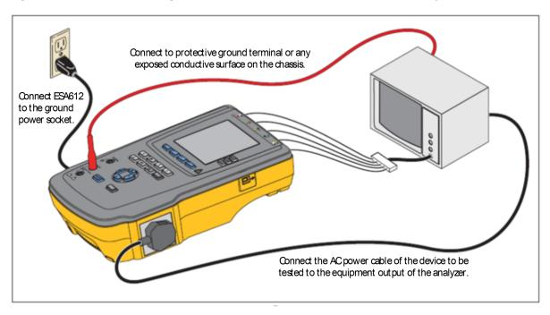
Figure3-5 Connection Diagram of the Device Under Test and the Analyzer
