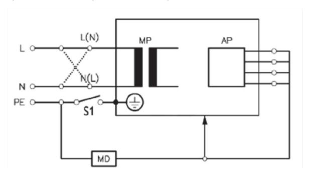
Figure3-4 Schematic Diagram of Device Leakage Current Test
