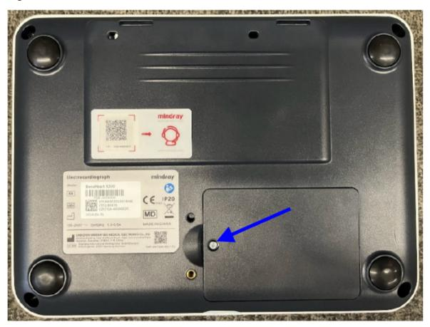
2. Loosen the battery cable buckle and remove the lithium battery. Press the recorder door button to open the recorder door, and then take out the printing paper. Use a screwdriver to unscrew the four M4×10 pan head cross recessed screws.
