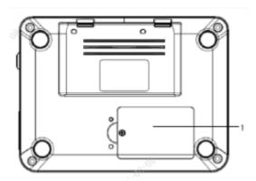
1 Battery compartment: Houses the battery for powering the device.
