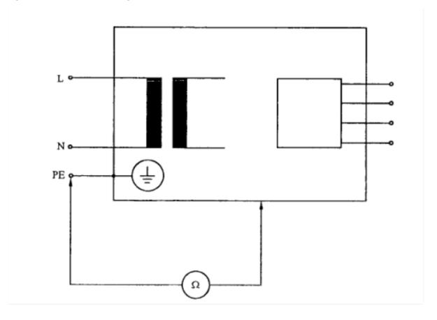
Figure3-2 Schematic Diagram of Ground Resistance Test
