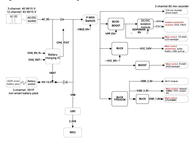
Battery of the host: R300 uses a non-intelligent battery with an output voltage of 9 V to 12.3 V.
