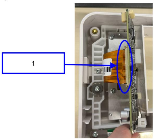
1 Loosen the socket and pull out the print head FPC cable.
