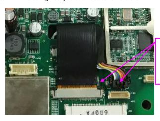
Open the receptacle clamp with tweezers and remove the two connection cables from
