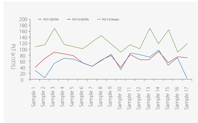
Figure 3: No dissociation effect of device B’s optical fluorescence platelet counting on EDTA-PTCP patients. PLT-I (EDTA), impedance platelet counts of EDTA-PTCP samples in EDTA tubes; PLT-O (EDTA), optical fluorescence platelet counts of EDTA-PTCP samples in EDTA tubes; PLT-I (citrate), impedance platelet counts of EDTA-PTCP samples in citrate tubes; EDTA-PTCP, ethylene diaminetetraacetic acid-dependent pseudo thrombocytopenia.
