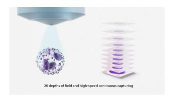
The MC-80 innovatively captures 20 images of each cell at different depths of field.
