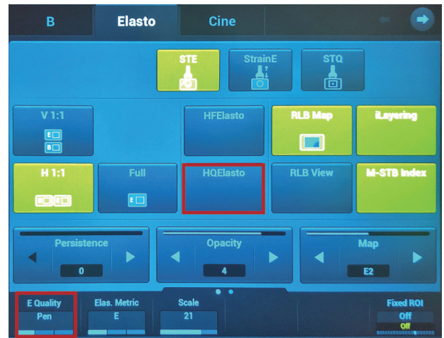
Figure 18. Image optimization options at the elasto panel of Resona 7 (red frames). The penetration, hence the reliability can be increased by switching E Quality to "Pen" and by activating "HQElasto" mode.
