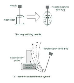
Figure 1. The schematic and principle of eSpacial Navi
