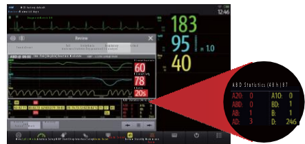
Figure 2: Statistical function for review of respiratory oxygenation (A20 refers to apnea lasting more than 20s, and A10 refers to apnea lasting more than 10s but less than 20s)
