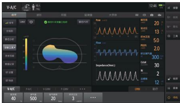
Figure: Ventilators with the integrated chest EIT feature
