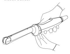
4. Inspect the sheath to ensure there is no hole or tear.
