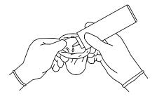
2. Insert the probe into the sheath; make sure to use proper sterile technique. Pull cover tightly over probe acoustic lens to remove wrinkles and air bubbles, and taking care to avoid puncturing the sheath.
