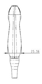
The above is a dimension illustration of the L14-5w probe. You can select the probe sheath according to the actual application situation.
