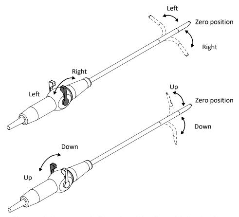
Figure 4-1: Laparoscopic Transducer Handle and Adjusting Levers
