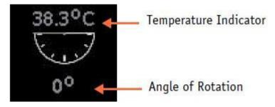
The angle of rotation shows the scan plane rotation while the temperature indicator shows the temperature at the transducer face. This indicator can optionally be turned off if the temperature is below 40.5°C. Above that temperature the indicator will always be displayed. In addition:
