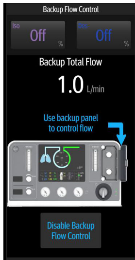
Figure 4-17 Backup Flow Control System
