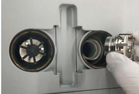
Figure 9-21 Insert the inspiration and expiration valves
