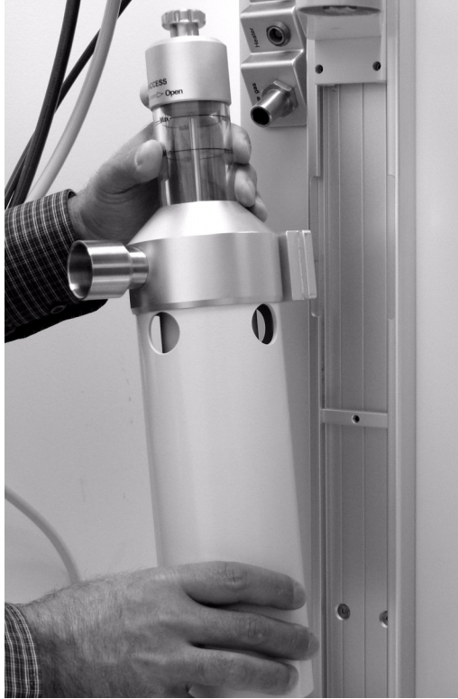
FIGURE 3-22 AGSS and Transfer Hose Removal
