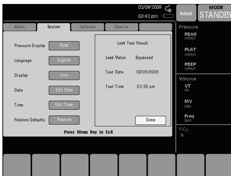
FIGURE 2-20 Example of a Bypassed Leak Test
