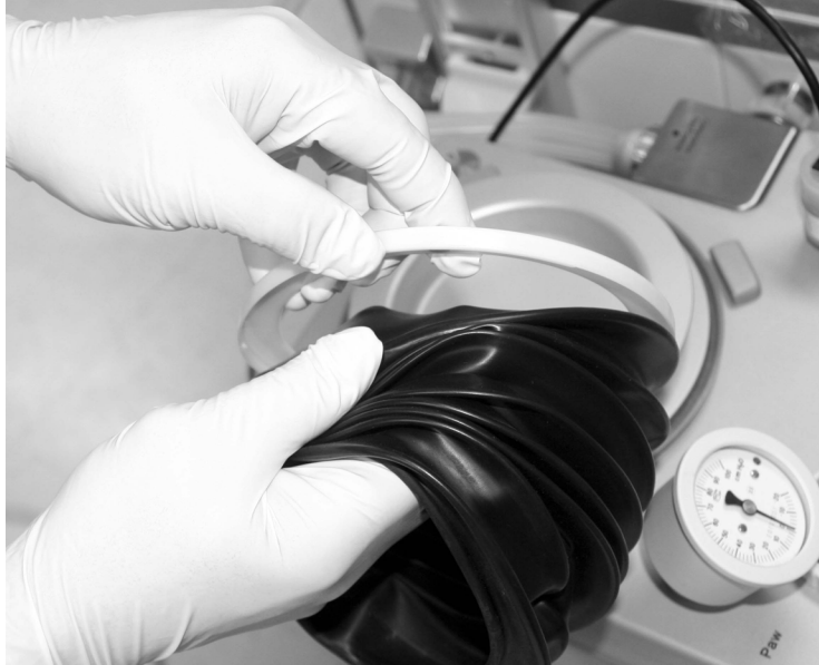
FIGURE 3-4 Detaching the Top Plate
