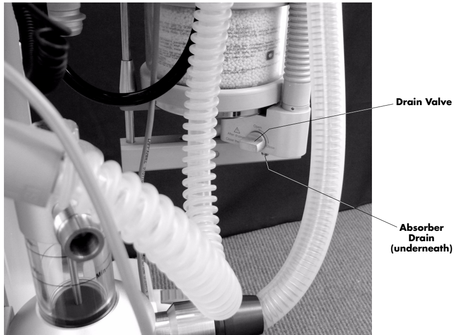
FIGURE 3-17 Absorber Drain Valve Location
