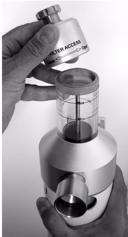
FIGURE 3-23 Removal of AGSS Top
