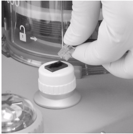
FIGURE 3-12 Oxygen Sensor External Cable Removal
