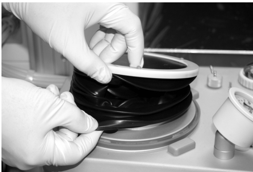
FIGURE 3-3 Detaching the Bellows
