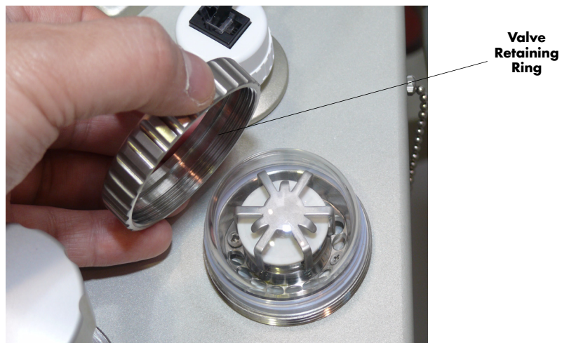
FIGURE 3-8 Valve Retaining Ring Removal
