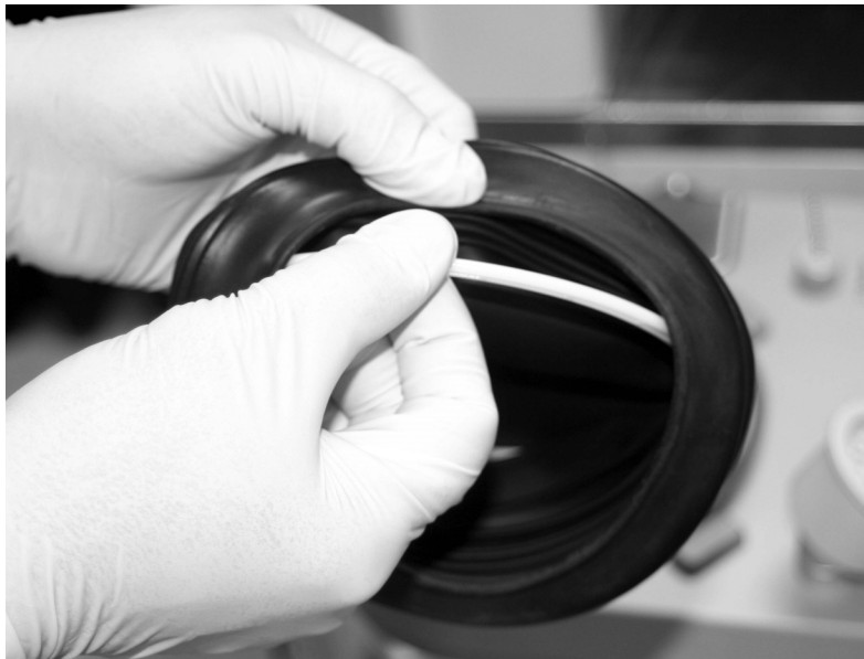
FIGURE 3-5 Removing the Bellows Adapter Ring
