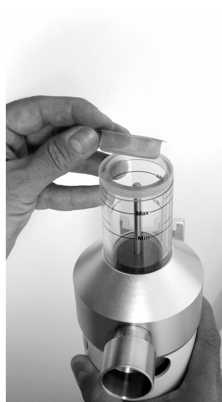
FIGURE 3-24 AGSS Filter Inspection
