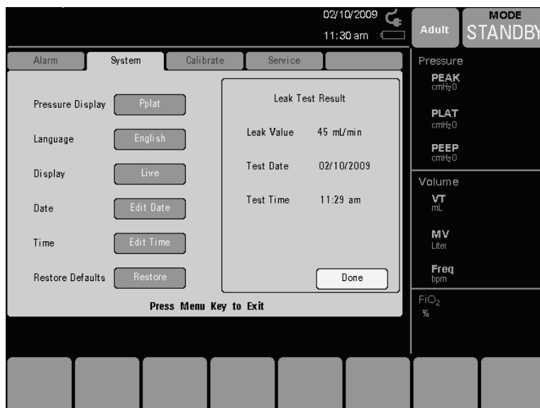
FIGURE 2-19 Example Leak Test Results
