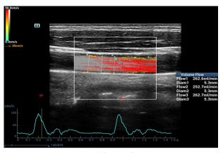
Fig. 9: Three measurements can be made for volume flow at the same image. The cardiac cycle is selected by VF and VF' in terms of the velocity curve as shown at the bottom of the image. Therefore, the volume flow is calculated according to one cardiac cycle based on vector flow velocities. The diameter is also shown along with the volume flow as presented in right middle of the image.
