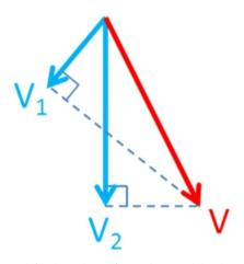
Fig. 3: Example for velocity obtained from two beams. Both the velocity and direction are obtained from an angle compounding technique, where V is the compounding velocity, and  $V_1$  are Doppler measured velocities.
