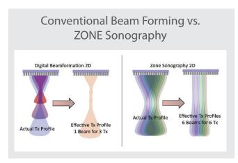
This proprietary method translates into a 2D image that is fully focused from skin line to deepest depth without the need for manual focal zone adjustment. Dynamic Pixel Focusing improves efficiency and the user-experience by reducing need for manual focal zone adjustments and providing a uniform image with improved spatial and contrast resolution throughout the entire field of view. Clinical benefits of Dynamic Pixel Focusing include:
