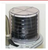
Remove the bellows dome by turning it counterclockwise and lifting it away from the breathing system.
