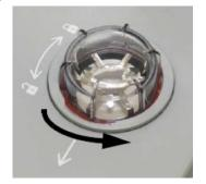
Remove the valve dome by turning it counterclockwise. Remove the valve from the breathing system.
