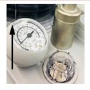
At the base of the bag arm, locate the retaining ring. Turn the ring counterclockwise until it is no longer threaded. Lift the bag arm from the breathing system block.
