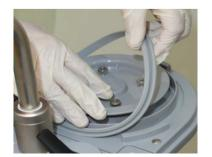
Remove the bellows dome O-ring.
