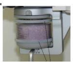
Rotate the locking mechanism handle clockwise into the unlocked position. Remove the absorber canister. Then remove the Pre-Pak or loose fill absorbent from the canisters. Dispose of the absorbent as per the local regulations.
