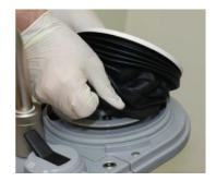
Detach the bellows from the base plate.
