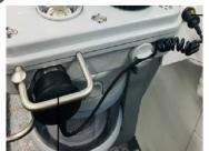
Disconnect the oxygen sensor cable from the main unit. Then hold the oxygen sensor and pull straight out firmly from the breathing system block. 9
