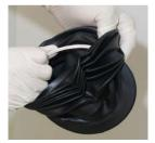
Remove the bellows adapter ring from inside the bellows. Note the orientation of the bellows adapter ring as it is being removed to ensure that it is properly inserted during reassembly. (If the ring contains grooves, the ring should be oriented so that the grooves are facing downward in the final reassembly.)
