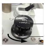
Loosen the base collar of the APL valve by turning the collar (not the valve knob) counterclockwise until it is no longer threaded. Then, firmly pull the APL valve upward to remove.
