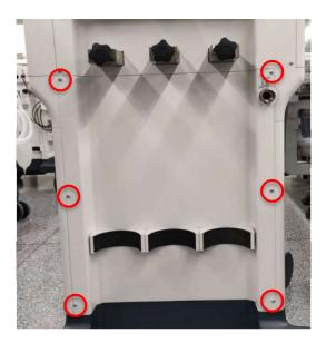
Remove the yoke panel: Unscrew the four screws on the upper rear panel (yoke cover) and pull it out.
