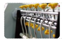
Bend-resistant cable, withstanding hundreds of thousands of bending tests
