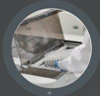
Up to 300 samples can be loaded and offloaded continuously
