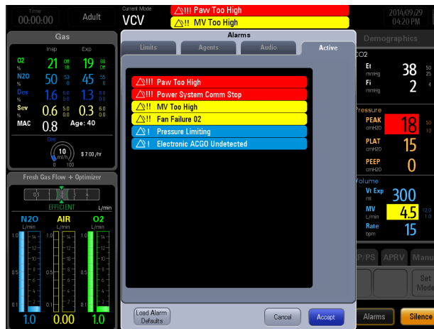
FIGURE 3-9 Alarm and Prompt Messages
