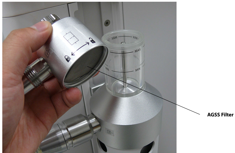
FIGURE 7-27 Removal of AGSS Top / AGSS Filter Inspection
