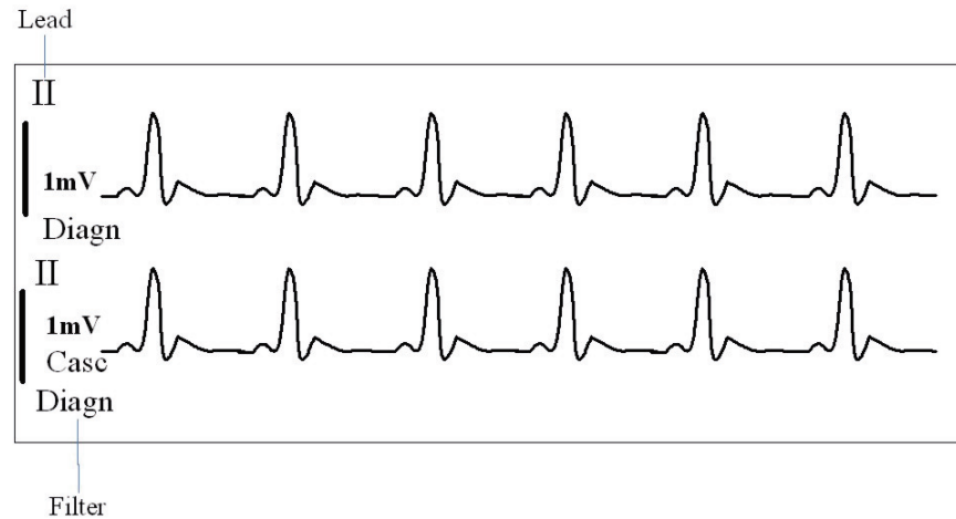
FIGURE 4-3 ECG waveform, 3-lead normal monitoring (cascade is turned on)
