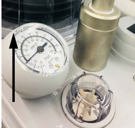
FIGURE 7-14 PAW Gauge Removal
