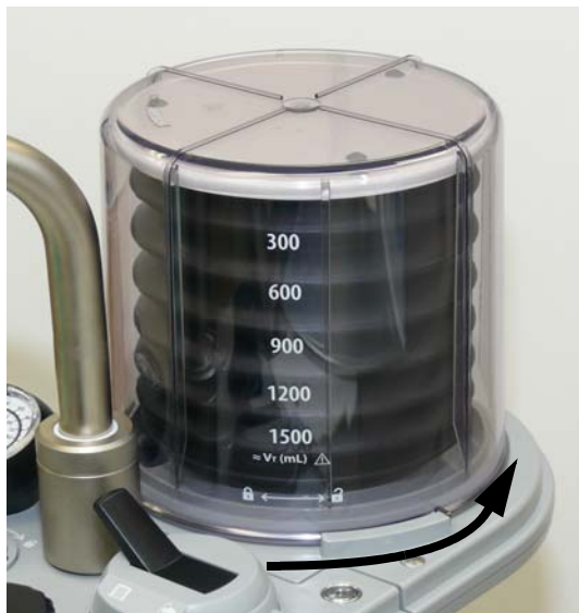
FIGURE 7-5 Removing the Bellows Dome
