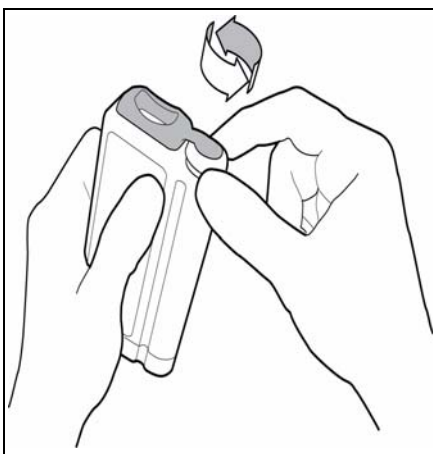
FIGURE 10-6 Removing Telepack-608 Battery Cap
