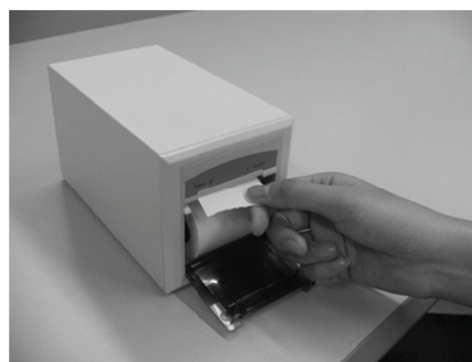
Figure 11-7 Installing Recorder Paper -3 Figure 11-8 Installing Recorder Paper -4
