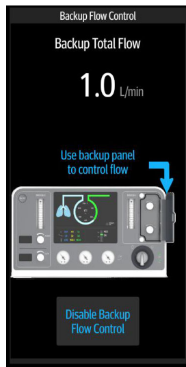
Figure 4-17 Backup Flow Control System
