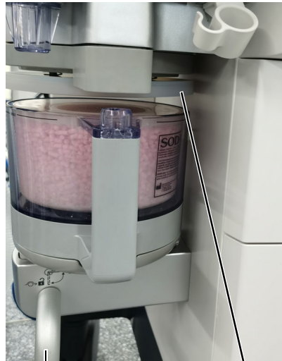
Unlocking position. The bypass is turned on.
