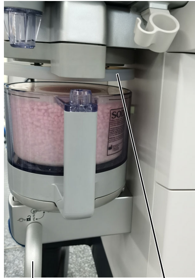
Unlocking position. The bypass is turned on.
