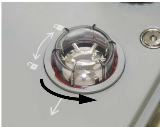
FIGURE 7-11 Valve Dome Removal
