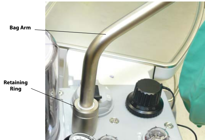
FIGURE 7-16 Bag Arm Removal
