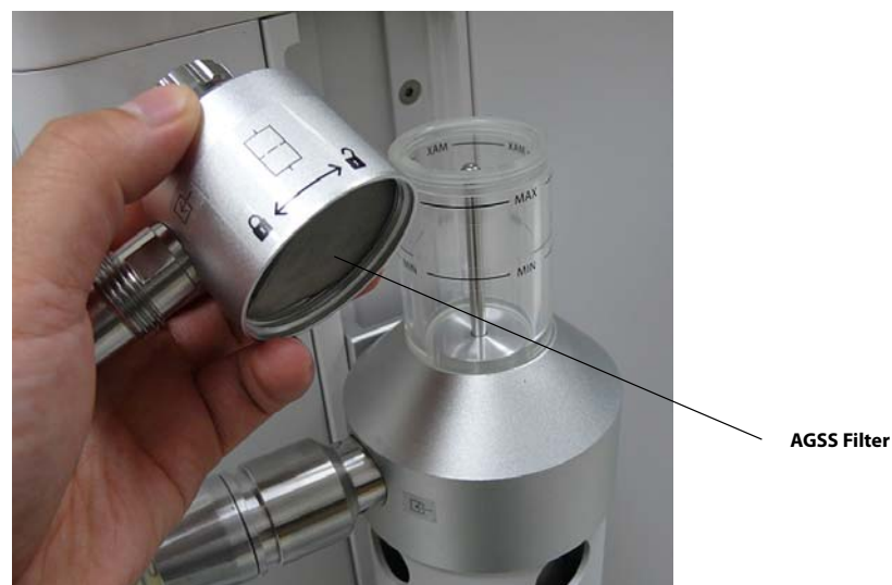
FIGURE 7-27 Removal of AGSS Top / AGSS Filter Inspection
