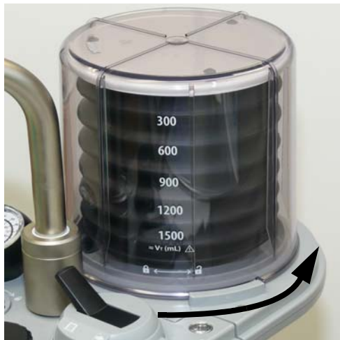
FIGURE 7-5 Removing the Bellows Dome
