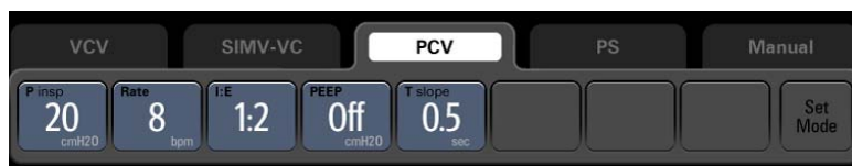
FIGURE 3-28 Ventilation Mode: PCV (A3 unit)
