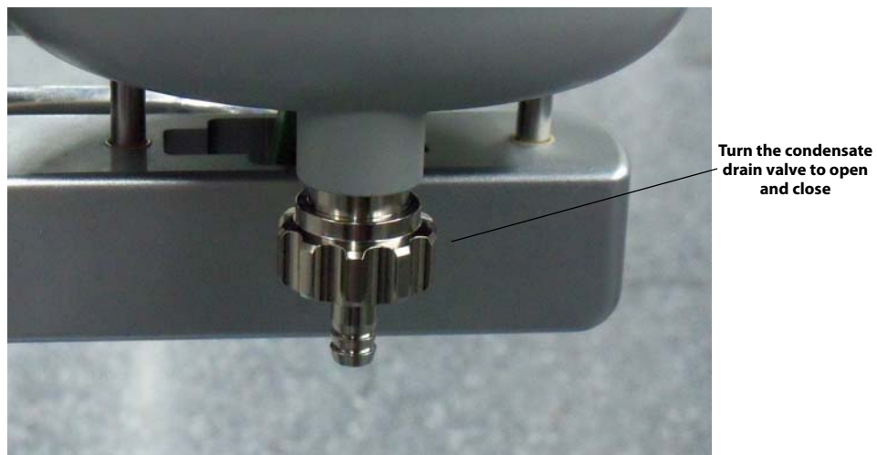
FIGURE 7-18 Condensate Drain Valve (Close Up View)
