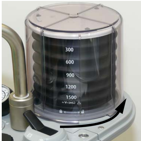
FIGURE 7-5 Removing the Bellows Dome
