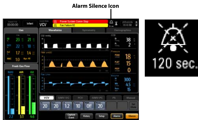
FIGURE 3-10 Alarm Silence Icon (with AG module connected)
