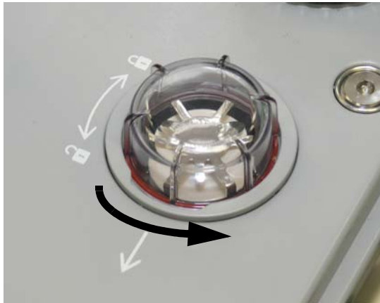
FIGURE 7-11 Valve Dome Removal
