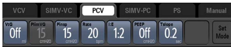
FIGURE 3-27 Ventilation Mode: PCV (A5 unit)
