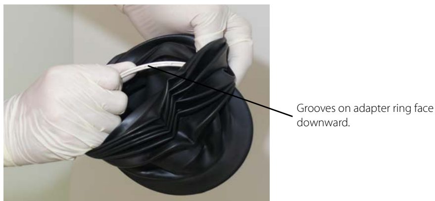
FIGURE 7-8 Removing the Bellows Adapter Ring
